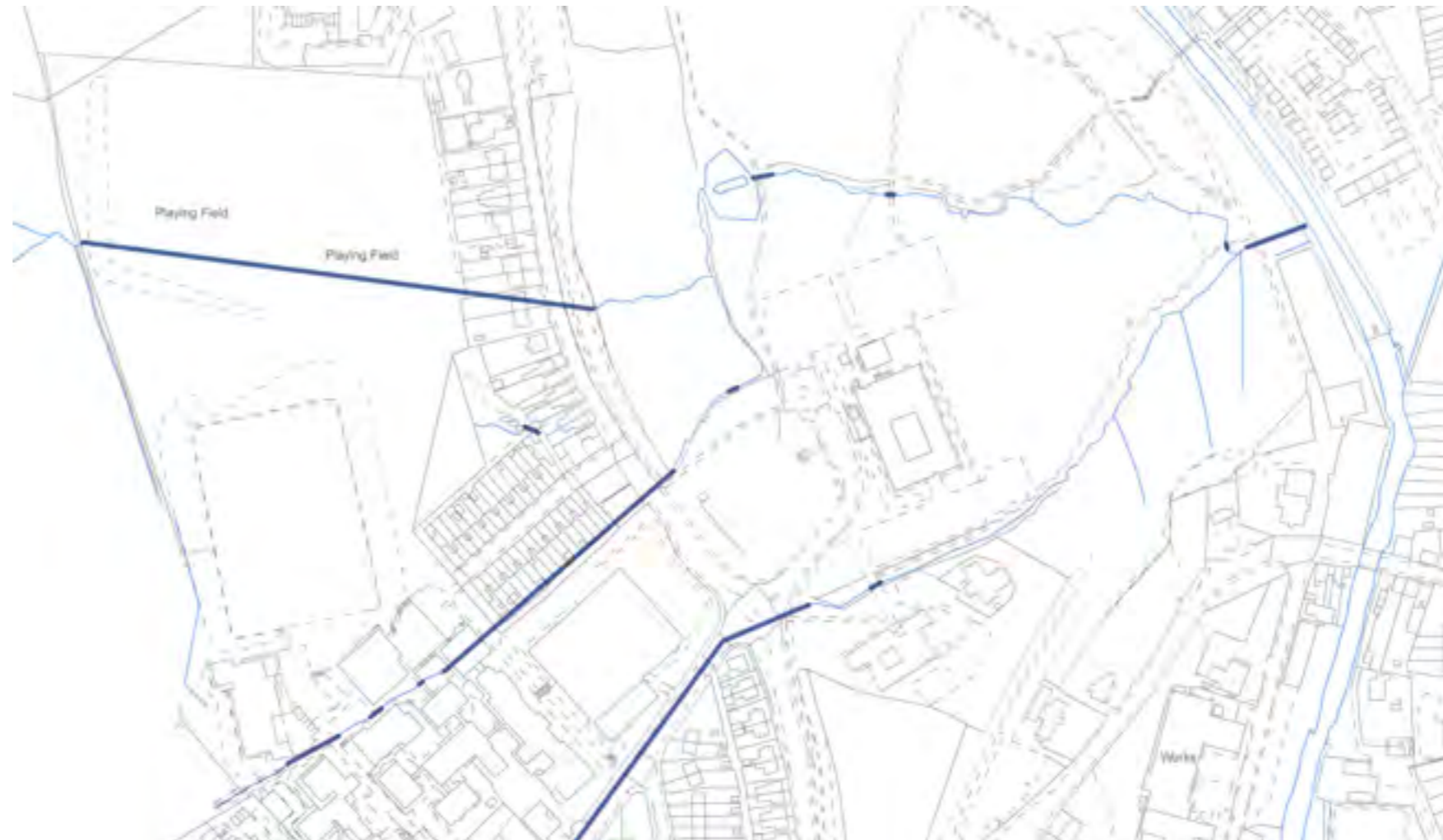
Figure 6: Culvert Plan (indicative culverted watercourses shown in bold) as provided by CCBC
