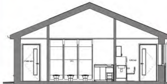
Typical Section Through Toilets 1:50
