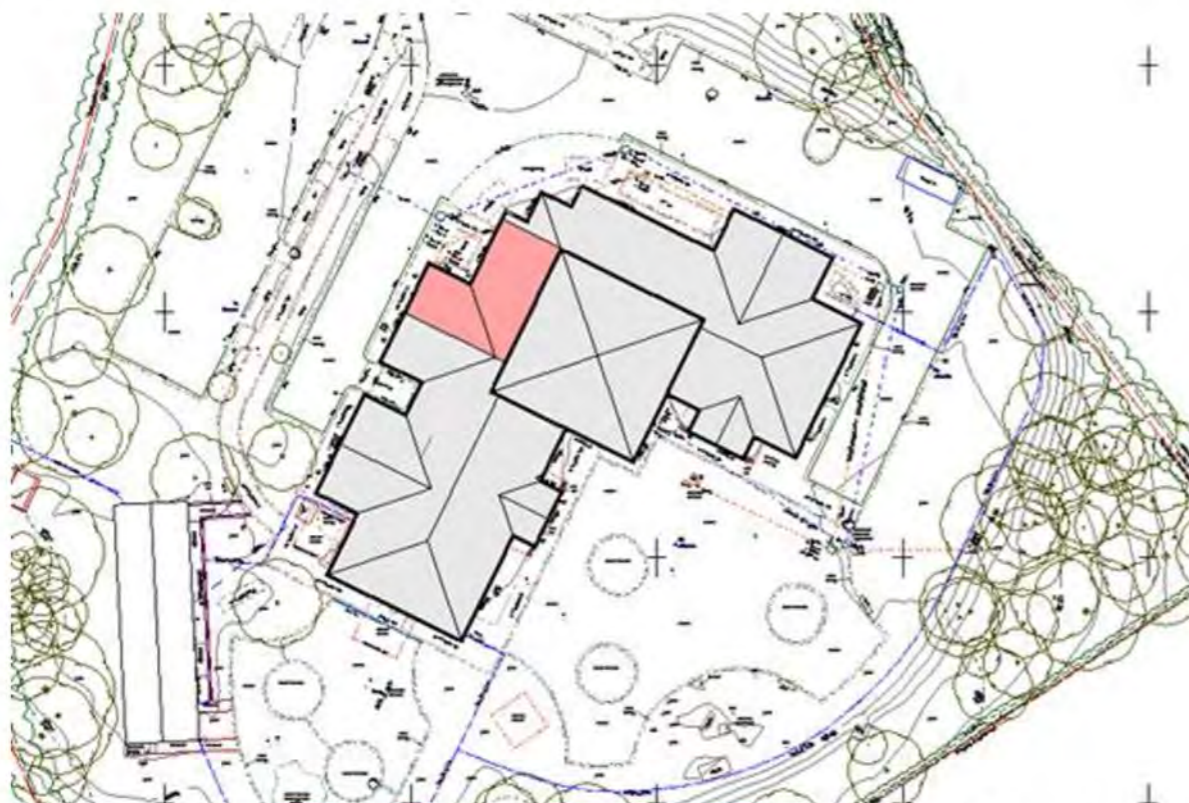
Figure 26 - The pink shading indicates the area of roof where alterations will be required in order to form a link to the new extension that will extend further west.
