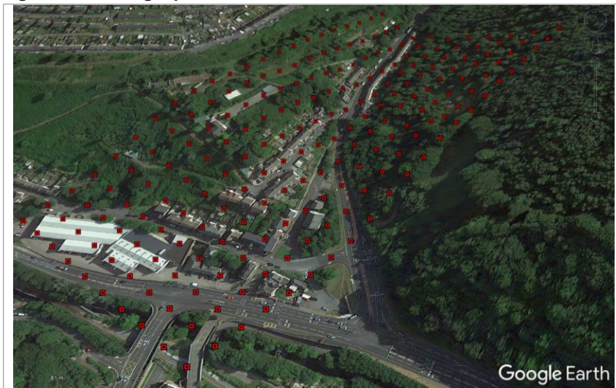
Figure 20: 200 height points used to build terrain model in GRAL
